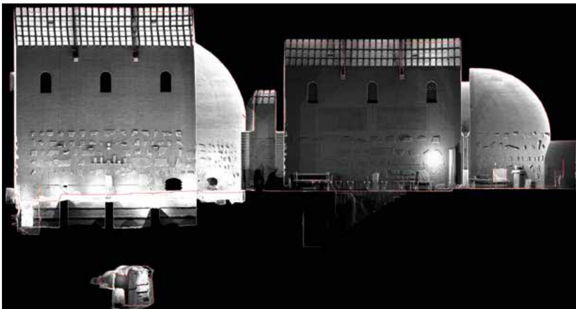
Fig. 4. Longitudinal section of the complex of the Basilica of St. Silvestro from the cloud of points Source Photographic Archives of the Pontifical Commission for Sacred Archaeology.
