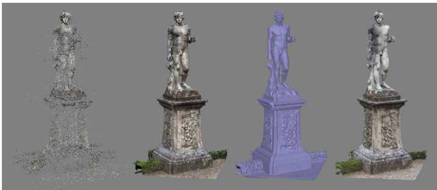
Fig. 4. The phases of reconstruction of the model. From the left to the right: sparse point cloud; dense point cloud; the mesh and the textured model.
