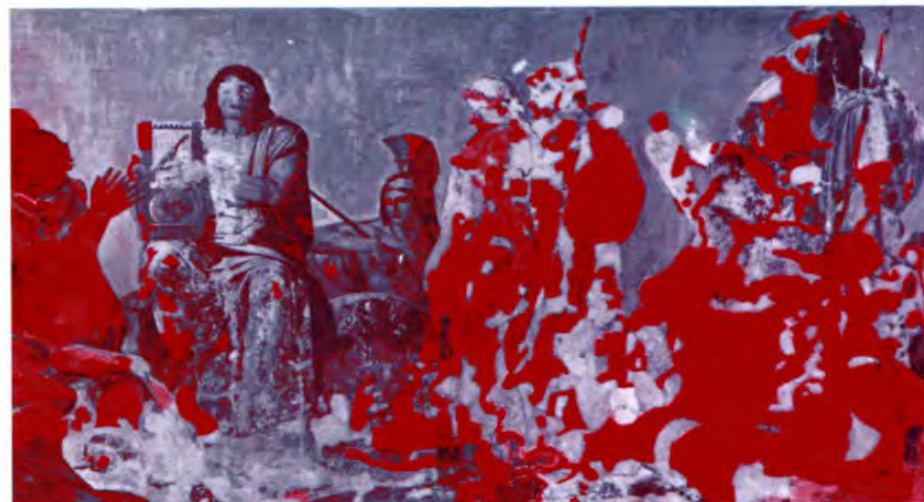
Figure 15. Munich, Ludwig-Maximilian University, lecture room no. 115, Ludwigstr. 28, R. V. Langer 1834, mapping of the salt efflorescence, foil on a black-and-white photograph, coloured pencil (detail).
